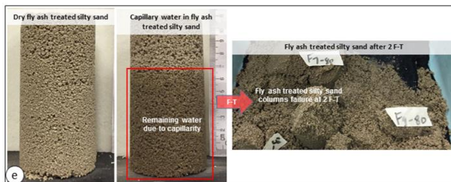
Figure 5.5 (continued) (e) F class fly ash treated silty sand soil columns
